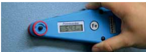
Figure 7: Coat thickness measuring of a ferrous surface (see Fe-designation).
