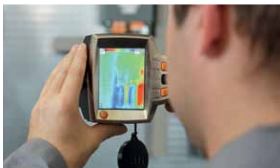
Figure 8: One testing method during the switch cabinet maintenance is to test the heat development of the electrical switching units.
